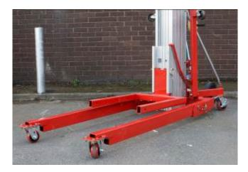
then insert the leg locking pins to secure the legs into the lift position.
