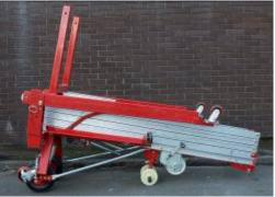
Position the material lift on a level surface, remove locking pins
