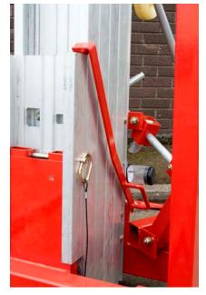
ALWAYS INSURE THE LOCKING ANCHOR AT THE BASE OF THE MAST IS SECURE BEFORE ATTEMPTING TO TRANSPORT OR MOVE THE MATERIAL LIFT TO THE HORIZONTAL POSITION.
