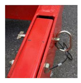
4, If the material lift is fitted with stabilising out riggers, please make sure these are lowered to come in contact with the floor.
