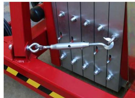
**IMPORTANT:** Replace the profile safety hook to stop the profiles from moving during horizontal transportation.
