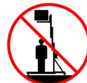
✓ Do not stand under or allow personnel under the **TORO** tower when the load is raised, making sure a safety area is blocked around the tower, which should have a diameter of 1.5 times the height of the tower.
