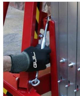
5.- Put the forks into the horizontal working position and lock them with the magnetic locking pins.
