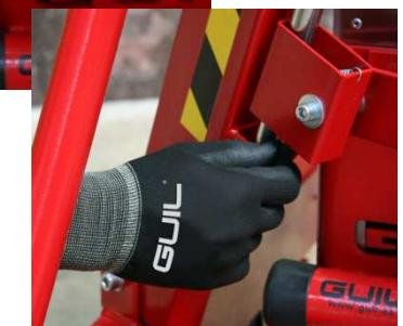
3.- Make sure the **TORO** is properly levelled using the spirit level as a reference. **VERY IMPORTANT:** At least 6 wheels must always be in contact with the ground.
