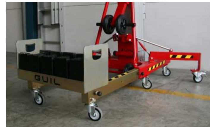
2.- Unfold the side stabiliser legs, starting with the leg with the sliding bar that is closest to the user (see pictures below).
