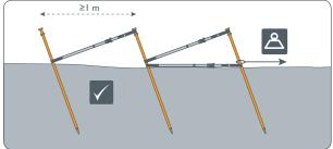
the first ground anchor stake, and the adjustable loop positioned at the base of the second ground anchor stake. Repeat for each subsequent ground anchor stake.
