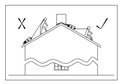
Figure 5 – Anchorage to minimise Fall Distance.
