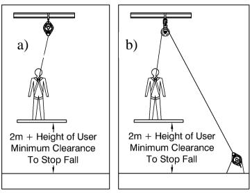
The anchorage for the G-Stop should be positioned so as to:
