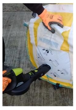
4. Insert the Inflator through the valve and inflate with the Inflator at maximum.
