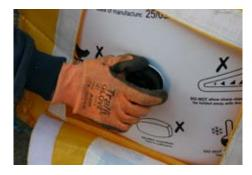
6. Once the liner is full of air, make sure the the nonreturn flap is securely seated and then screw the cap on tightly.
