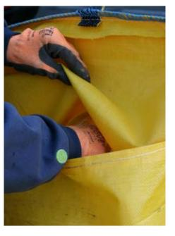
8. Should this not be the case, deflate the liner slightly and adjust by pulling the liner through the access overlap flap at the far end of the liner.
