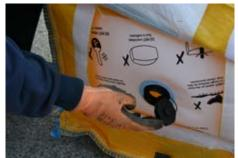
11. To deflate the bags remove the valve screw cap. Push back the flap using the red tab until it locks in position. Using the extract facility on the pump, if it has one, draw out all the air. Alternatively the bags will deflate rapidly if the valve is just left open.
