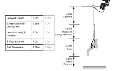
During a fall the energy absorber may deploy by up to 1.65m. Allow sufficient clearance between the anchor point and the ground or anything else below. heighter reccommend a clearance of 7.0m for 2m lanyards.
