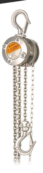
With a weight of 2.4 kg, a minimum height of 217 mm and a load capacity of 250 kg, the KITO CX003 manual chain hoist is one of the smallest and lightest manual chain hoists available. Followed by CX005 with a weight of 4.5 kg, minimum height of 260 mm and 500 kg load capacity.
