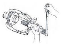
2. Tighten clockwise the Control valve knob
