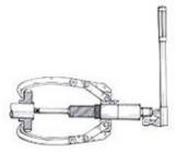
3. Center the Movable Cone in the object to be pulled. Then adjust the lock nut and jaws to proper position.
