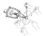
6-1. 360° Rotary pump handle, very easy to locate in the most convenient pumping position.
