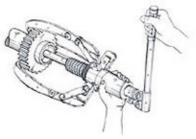
6-2. Loosen the Control valve knob to allow the Movable Rod return for next use.
