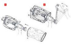
4. Important Notice: Before operating this unit, insure putting the safety net on(refer to the above)and covering the whole object completely.
