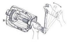
5. One hand holds the Puller; the other pushes the handle up and down till the object is pulled out.
