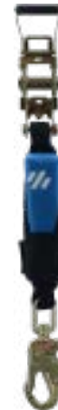
Integrated tear pack limits forces being put through anchor points to below 11kn
