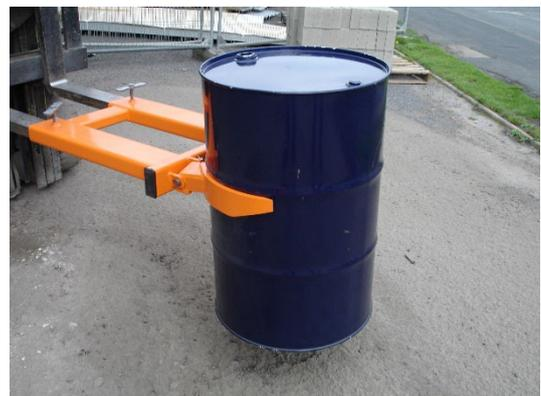
**If your drums are damaged, open topped, or empty you will experience difficulty lifting with this attachment. The IRG range are best suited for lifting this variety including straight sides drums.**
