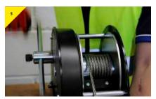
Release the cable tensioner and wind on the cable carefully by rotating the handle in a clockwise direction.
