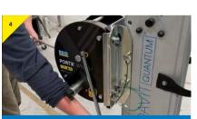
Note: The mechanism will only be active as long as the lever is held in the active position
