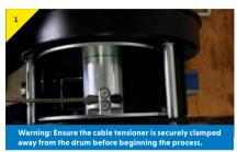
Locate the wire rope clamp on the drum and feed the end of the cable through the inner clamp location.
