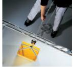
**Safety under control:** The Yale*lift*  $360^\circ$  for heavy industrial applications and will revolutionise every operation. By means of the  $360^\circ$  rotating hand chain guide, the user can operate the hoist from all directions and is no longer directly within the danger zone as before.
