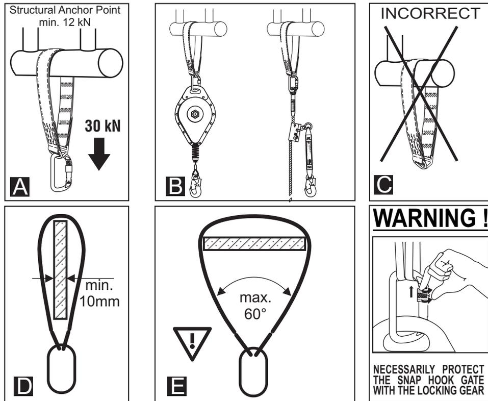
The Anchor Device can be put around a beam of different shape made of concrete or metalurgical rolled section
