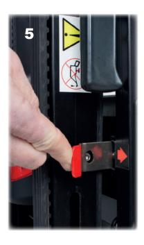
Pull out the track assembly using the top black bar, figure 6
