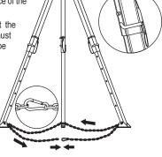
During the installation of the cable on the head of the deployed tripod head it is possible to step onto the tripod leg using the steps. They are installed on the outside of the legs in the holes used for adjusting the height of the tripod.
