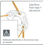
The Edge Guard must be positioned so that the rope runs over the centre of the Edge Guard, and does not lift out or become trapped against the side plates. Use the Velcro tabs to help keep the rope in place.
