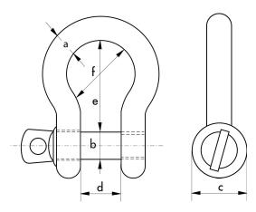
Material 17/4 PH precipitation hardening martensitic stainless
