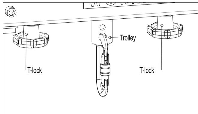
For safety trolleys SHOULD BE always positioned.
