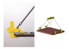
Warning! Some types of clamp are designed to be used with an endless loop of chain and others are for use with a two-leg sling. Under no circumstances must an endless loop be substituted for a two-leg sling or vice versa as this will alter the geometry and therefore the gripping forces on which the clamps rely for their safe operation.
