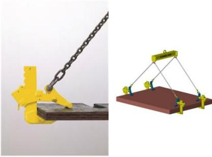
**Warning! Some types of clamp are designed to be used with an endless loop of chain and others are for use with a two-leg sling. Under no circumstances must an endless loop be substituted for a two-leg sling or vice versa as this will alter the geometry and therefore the gripping forces on which the clamps rely for their safe operation.**
