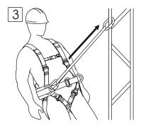
ATTENTION: Make sure that connections between each separate fastening element are stable prior to commencing work and while working. Snap hooks must be closed and protected with a mechanism which prevents them from accidental opening.
