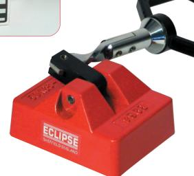
The Steel Plate Drag is used to remove ferrous steel sheets and plate from a stack and for transporting ferrous sheets and plates to and from machines. The lever can be positioned to operate a quick release mechanism to force the Steel Plate Drag to push the steel sheet or plate off the magnetic clamping surface.
