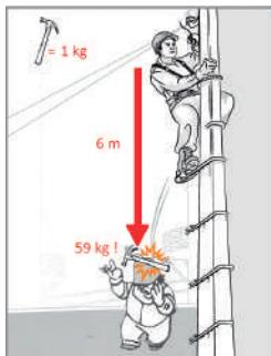
The S-Tools Systems range was developed to hold any type of tool that may accidentally fall. In fact, objects dropped by workers are the second largest cause of worker deaths in the workplace. The consequences of a falling object are often underestimated. Dropping a work tool also means the risk of destroying the tool, and possible damage to property can also have serious consequences in terms of costs, as well as lost time when workers leave their work station to retrieve their tool.
