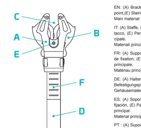
EN: (A) Brackets, (B) Legs, (C) Gate, (D) Attachment point, (E) Stainless steel pins, (F) Main stitch.
