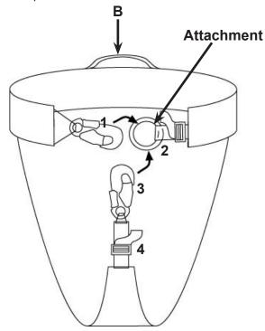
Step into harness, fasten and adjust in the order shown in the diagram above, 1,2,3,4 (Class B).
