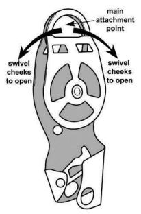
For use only with 10.5mm to 11.0mm diameter low-stretch rope.
