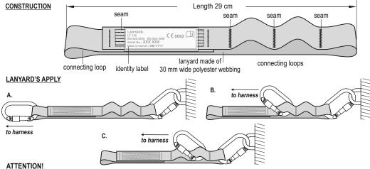
The lanyard can be equipped only with certified snap hooks according to EN 362.
