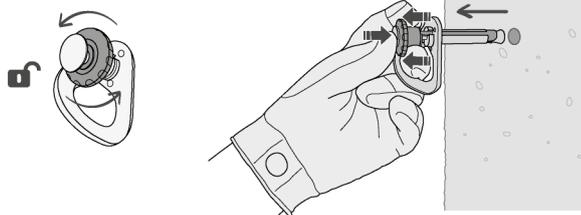
5. Installing the anchor
