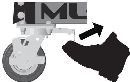
9. Lay the machine down in front of the loading ramp of the trailer or low loader so that the braked swivel castors and loading wheels are in contact with the ground, and the hoisting anchor on top of the mast is facing the loading ramp.
