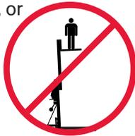
**NEVER** operate a ToughLift® Material Lift in the vicinity of live electric conductors as the machine is not electrically insulated.
