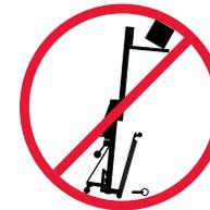
**NEVER** move a ToughLift® Material Lift when the carriage is loaded, whether the mast is lowered or raised (except for very minor repositioning).
