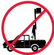
**NEVER** raise the mast (loaded or unloaded) unless all 4 (or 6 if stabilisers are fitted) castors are in touch with the ground.
