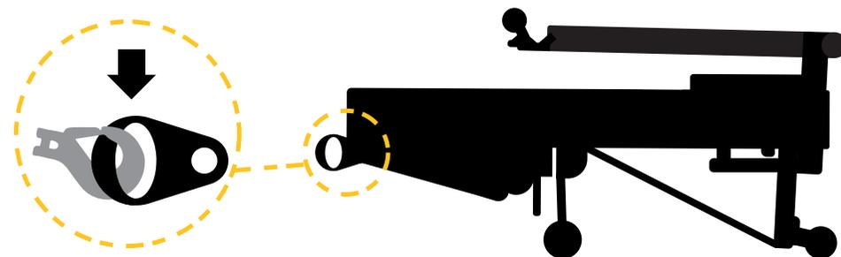
11. Winch the machine up onto the trailer or low loader.
