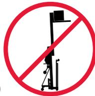
**NEVER** operate a ToughLift® Material Lift in strong or gusting winds. The larger the surface area of the load being lifted, the greater the effect of wind on the stability of the machine.
