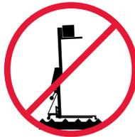
**NEVER** raise the mast (loaded or unloaded) unless the front legs and stabilisers (if the model being used is equipped with stabilisers) are deployed and locked in position.
