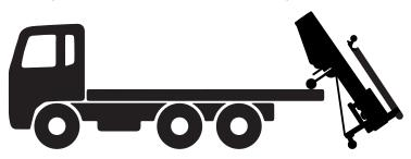
9. Use a minimum of 2 straps or chains to secure the machine to the flatbed of the vehicle or trailer. If laying the machine down on the vehicle or trailer, ensure that the straps are placed over the mast, as putting them over the front legs could cause damage to the machine.
