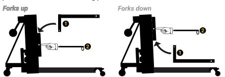
b. Load Platform: Place the Load Platform on the Standard Forks (forks up or forks down) with the 2 locking tabs facing down at the carriage end of the Standard Forks.
