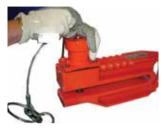
Remove the 4 No. M8 cap head screws holding the tube assembly to the shackle body.
