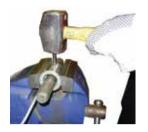
The sleeve can now be replaced and coiled pin hammered back in place. A new coiled pin may be required if the old one is damaged.
