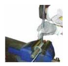
Drive the coiled pin out using a 5mm punch.
