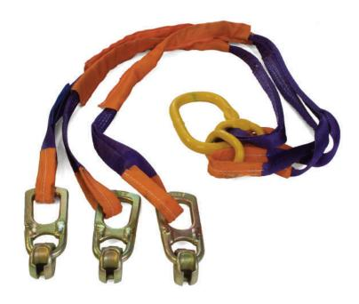
The Pin Anchor Sling Set is a robust lifting devise manufactured from several cast components. The lifting clutch is designed to fit only the Pin Anchors and Recess Formers for the chosen load category. This in built safety feature, ensures that mismatching of load groups cannot occur.
