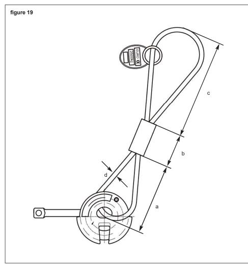
The Spread Anchor Combination Ring Clutch is similar in specification to the standard Spread Anchor Ring Clutch, but supplied with a wire rope lifting chain attachment. The wire rope offers greater flexibility when lifting elements with edges that may come into contact with the clutches chain attachment link. Minimising the potential cosmetic damage of the concrete.
