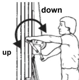
**Test Two-Speed Winch Operation**
